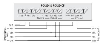
Note: for this option, Jumper J1 must be set for 'Combus Relay'
