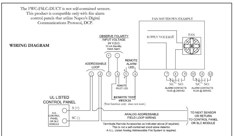
**CAUTION:** Since the analog loop is current limited similar to a conventional two-wire loop, the FWC-FSLC-DUCT cannot be guaranteed to operate under all conditions. This analog duct housing must be treated as a two-wire conventional duct detector when considering auxiliary functions necessary for smoke control.
